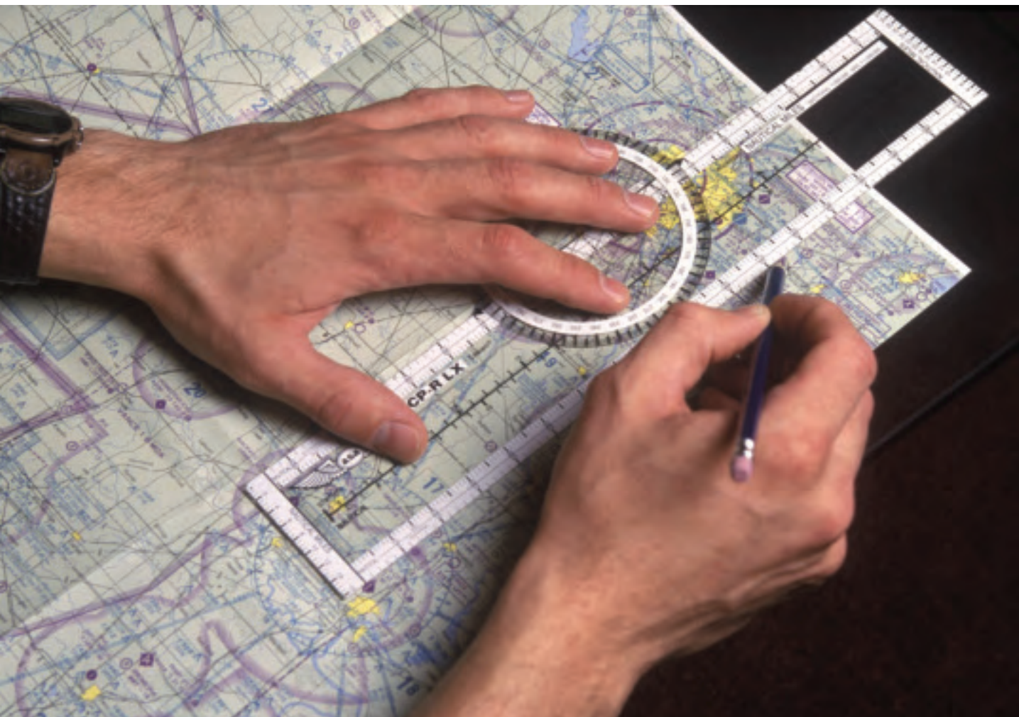
A student pilot uses a course plotter to mark a flight path.
