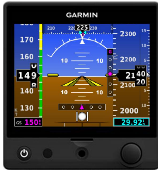
Figure 1-1, G5 Electronic Flight Instrument (Attitude)
