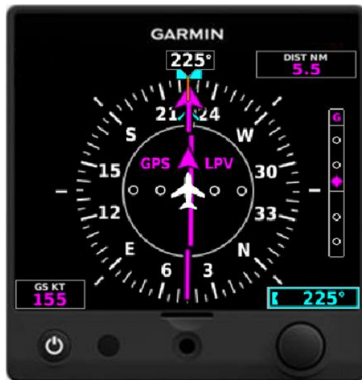
Figure 1-3 G5 Electronic Flight Instrument (DG/HSI)
