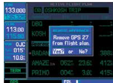
To remove an approach, departure or arrival from the active flight plan, highlight the procedure name (appears in light blue text) and press CLR.
