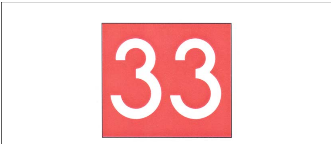
FIG 2-3-25 Holding Position Sign at Beginning of Takeoff Runway
