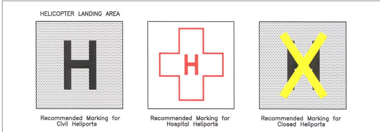
FIG 2-3-23 Helicopter Landing Areas
